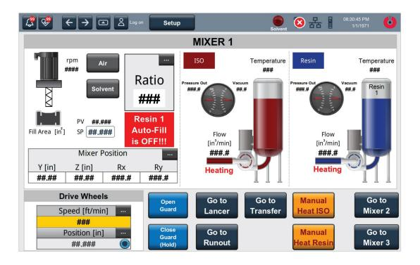
The Fillameter HMI is equipped with a 12" Allen-Bradley 5310 touchscreen interface with a movable arm.
