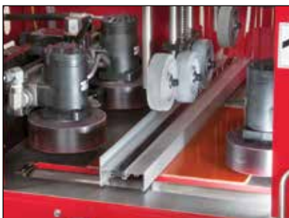
MLP™ (mechanical lock profile) with large debridge gap
