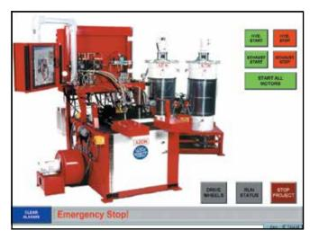
All motors start and stop from the main screen including the hydraulic power unit, fume extractor and chemical agitators.
